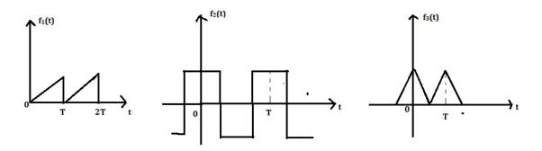
The fundamental frequency of the periodic signal is given by  $\omega_o=2\Pi/T$ . If 'n' is any integer, then  $n\omega_o$  is called  $n^{th}$  harmonic of the fundamental frequency  $\omega_o$ .
